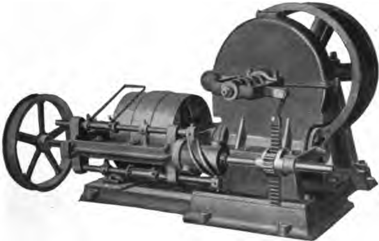
Fig. 41. Floor Type of Worm-Gear Machine with Cylindrical-Cam Belt Shipper
